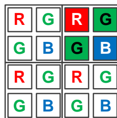
Figure 8-48 Horizontal and vertical color Binning by 2x2
